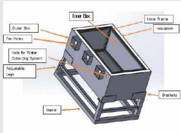
Demonstration of the original prototype operation and design
